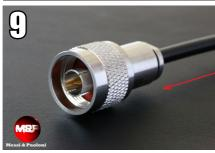
Insert the connector and fasten accurately until the o-ring present in component A, will be pressed against the connector body. Inside, the rubber component C (pic. 1) will expand, granting optimal sealing against moisture and a perfect contact to ground.
