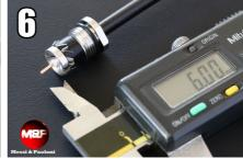
Cut and remove the tape and dieletric for a lenght as shown in the picture (in mm).
