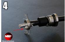
Insert component D after having opened the braid as shown in the picture. Push component D between the foil and the braid until it stops against the red PE jacket.
