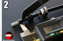
Insert in the cable components A, B, C and immediately after, make a circular cut on the red PE jacket at the indicated length shown in the caliber (in mm). Subsequently remove it.
