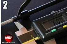
After having made the first cut, as shown in picture 2, rotate the cable 180 degrees and make a second cut in the same way, in order to facilitate the introduction of component D (pic.3 and 4)
