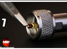
Fasten together the connector and component A, until it will be pressed against the connector body. Inside, the rubber component C (pic. 1) will expand, granting optimal sealing against moisture and a perfect contact to ground.
