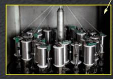
High resistance screen made of a sturdy copper **BRAID** (Cu). The braiding process is operated by means of **24 spools** braiding machines. (50% more crossings if compared to traditional 16 spools machines). Highly effective against low frequency impulsive noises.
