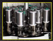
Screen made of a sturdy Aluminium-Magnesium alloy BRAID (AIMg). The braiding process is operated by means of 16 spools braiding machines. The braid plays an important role against low frequency impulsive noises.
