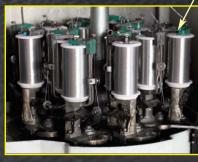
High resistance screen made by means of a sturdy Aluminium-Magnesium alloy **BRAID**. (**AIMg**). The braiding process is operated by means of **16 spools** braiding machines. Highly effective against low frequency impulsive noises.
