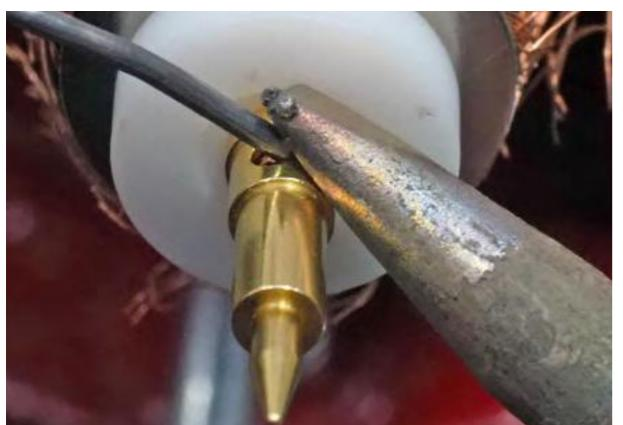
The welding must be as quick as possible: 2-3 seconds for "N" connectors.
