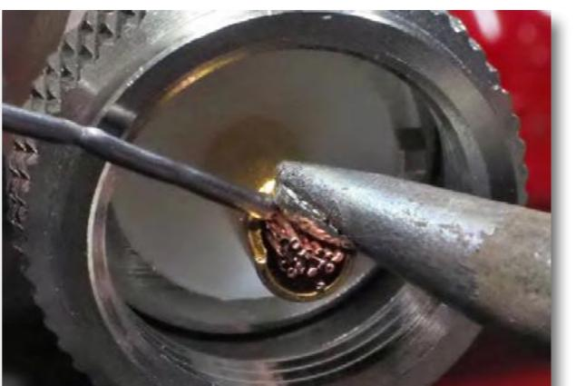
To fill the cavity of the "UHF" connectors repeat the welding in 2-3 times by adding tin every time.
